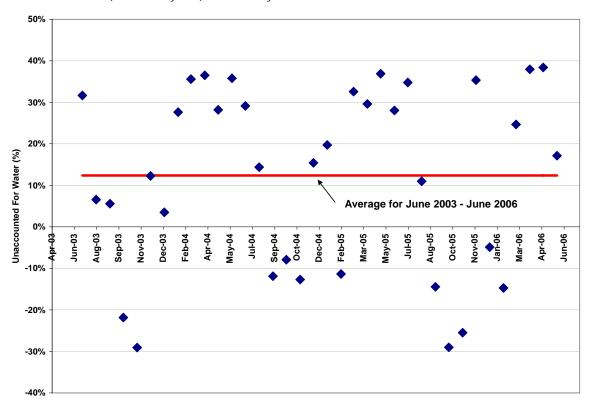
EXHIBIT 4-19 Unaccounted-for Water for 2004 and 2005 *Redmond Wastewater (Collection System) and Water System Master Plan*
